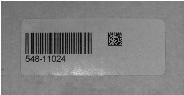
Fig. 267: Comparison of DataMatrix code and barcode
