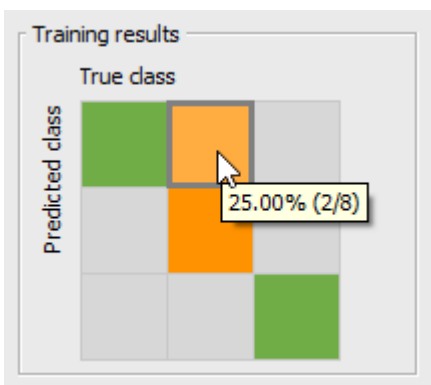
Fig. 206: Training results - 25% detected incorrectly
