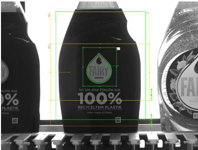
Fig. 262: Case 1: Label correctly applied
