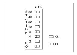
Use the head station switches to set the station number for addressing this slave station in the PROFIBUS/DP.
