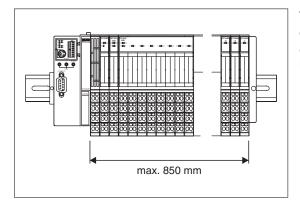
The maximum width of a station consisting of modules of the MELSEC ST series is 850 mm. Please note that the width of the head station is not counted.
