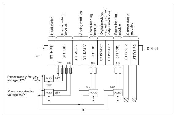
The DIN rail on which the modules are mounted must be conductive.
