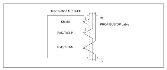
If the head module is the last station in a branch, then the PROFIBUS/DP line must be terminated with resistors. For the PROFICON-PLUS and PROFICON-PLUS PG plugs the resistances are already installed and can be switched on. For a plug without integrated resistors, three resistors must be connected according to the following circuit diagram. The resistors are not included in the module's scope of delivery.
