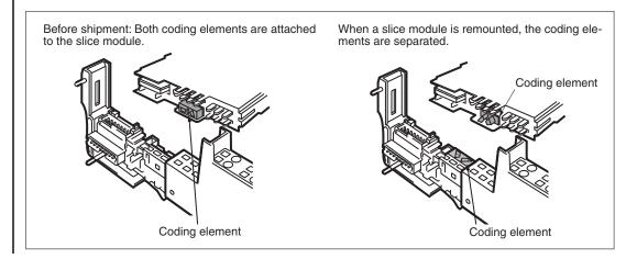
Do not use excessive force if an electronics module cannot be inserted in a base module. In this case, check whether a code element is already installed in the base module.
