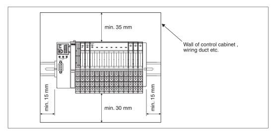
When mounting, please pay attention to alignment of the modules to ensure adequate ventilation:
