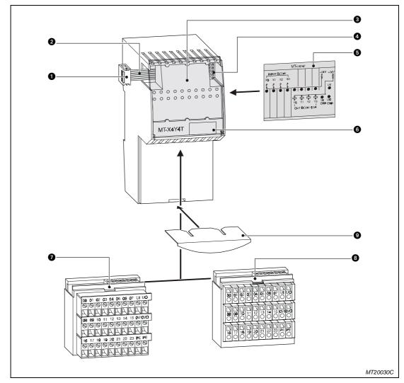
Fig. 4-26 shows the operating items and accessories of the MT-X4Y4T module (4 digital inputs, 4 transistor outputs):
