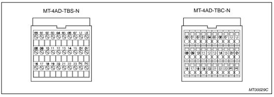
Fig. 4-31: Terminal blocks MT-4AD-TBS-N and MT-4AD-TBC-N
