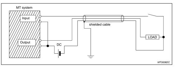
Fig. 5-17: Wiring and grounding of the I/O signal line
