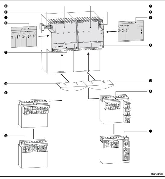
Fig. 4-22: Digital output module MT-Y8R5
