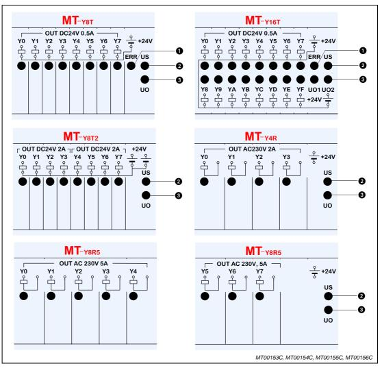
Fig. 9-5: Diagnostics indicators on digital output modules
