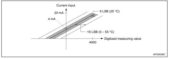
Fig. 4-41: Overall accuracy of the current input characteristics (4 – 20 mA)
