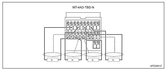
Fig. 4-53: Sample connection for the current output
