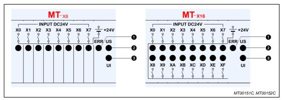
Fig. 9-4: Diagnostics indicators on digital input modules
