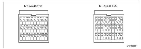
Fig. 4-27: Terminal blocks MT-X4Y4T-TBS and MT-X4Y4T-TBC
