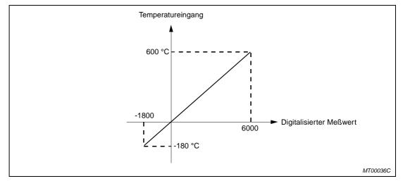
Fig. 4-38 shows the graph of the temperature input characteristics:
