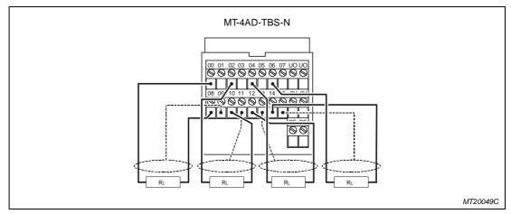
Fig. 4-51: Sample connection for the voltage output (-10 V – +10 V)
