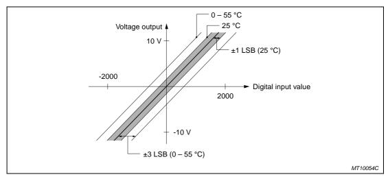
Fig. 4-55: Overall accuracy of the voltage output characteristics
