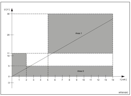
Fig. 10-1: Characteristic curve areas IEC 1131-2, type 2
