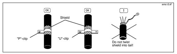
Abb. 5-13: Cable routing and shielding via "P"-clip or "U"-clip
