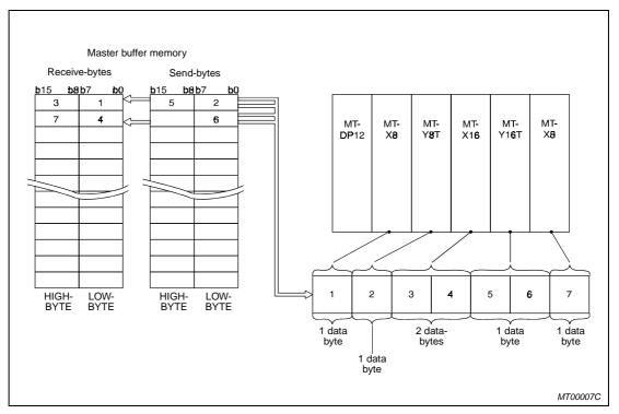
Fig. 3-8: Incorrect installation order
