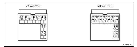
Fig. 4-21: Terminalblocks MT-Y4R-TBS and MT-Y4R-TBC
