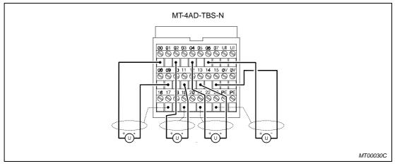
Fig. 4-32: Sample connection for voltage measurement
