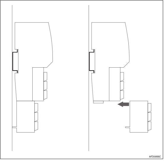
Fig. 5-8: Mounting potential terminal block
