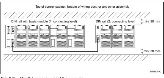
Fig. 5-2: Parallel arrangement of the modules
