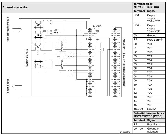
Tab. 10-16: External connection of the MT-Y16T module
