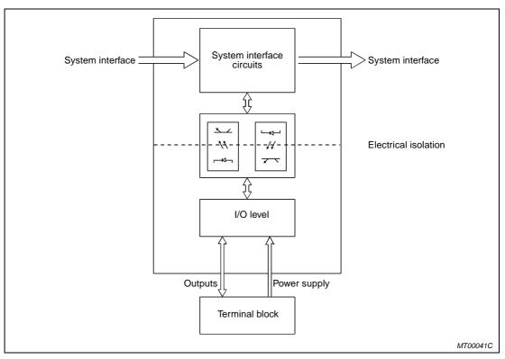
Fig. 4-43: Block diagram of the analog output modules
