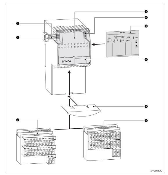
Fig. 4-49 shows the operating items and the accessories of the MT-4DA module:
