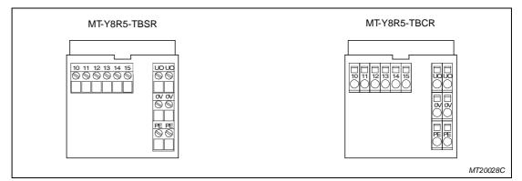
Fig. 4-24: Terminal blocks MT-Y8R5-TBS and MT-Y8R5-TBC
