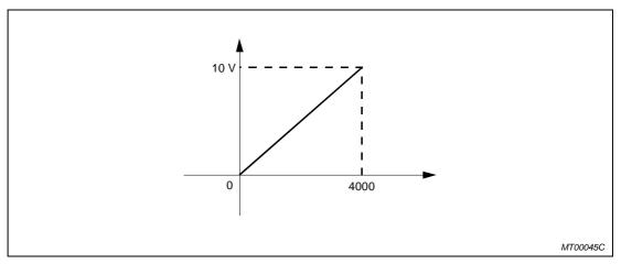
Fig. 4-47: Voltage output characteristics
