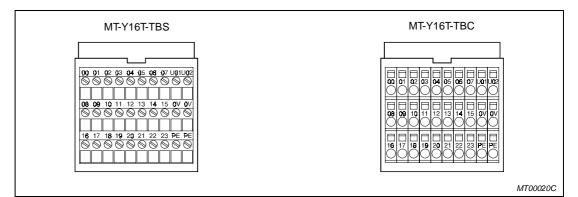
Fig. 4-16: Terminal blocks MT-Y16T-TBS and MT-Y16T-TBC
