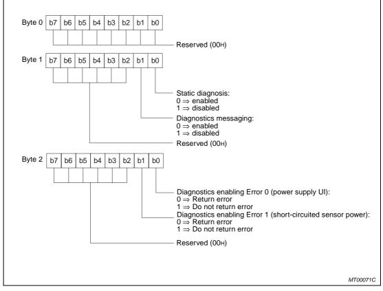
Fg. 7-2 shows the parameter arrangement of the MT-DP12E module.
