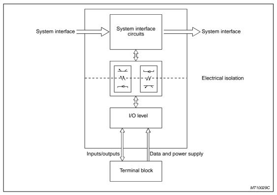
Fig. 4-25: Block diagram of the digital input/output modules
