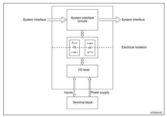
Fig. 4-6: Block diagram of the digital extension modules
