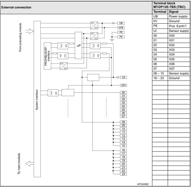
Tab. 10-8: External connection of the MT-DP12E module
