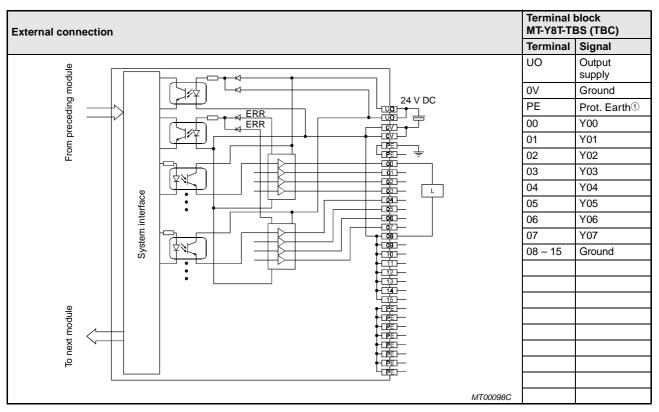
Tab. 10-14: External connection of the MT-Y8T -module
