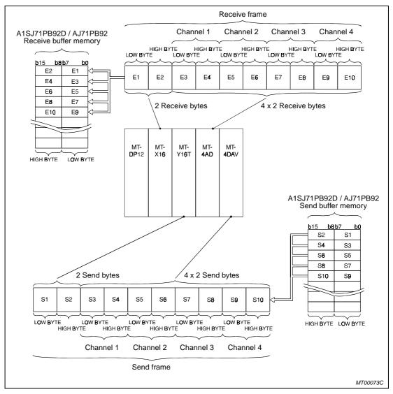
*Fig. 7-4:* Receive and send sequence of the protocol frame bytes
