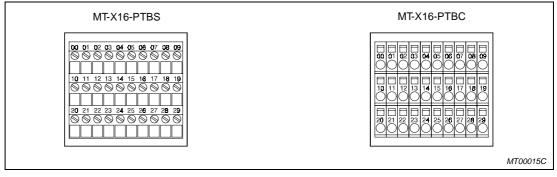
Fig. 4-11: Potential terminal blocks MT-X16-PTBS and MT-X16-PTBC
