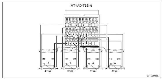
Fig. 4-37: Sample connection for PT100 measurement
