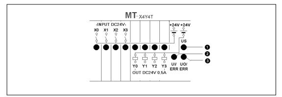
Fig. 9-6: Diagnostics indicators on digital input/output modules
