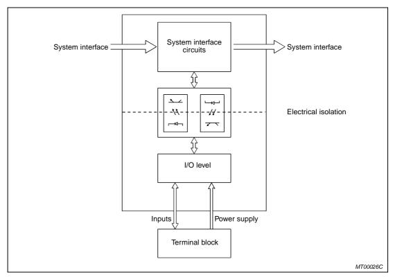
Fig. 4-28: Block diagram of the analog input module
