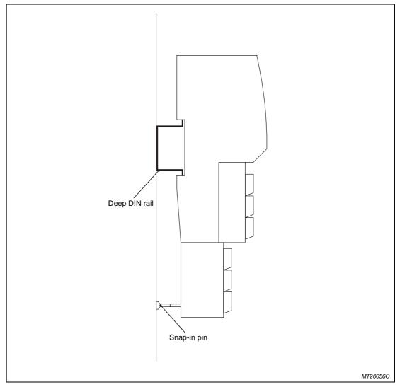
Fig. 5-9: Mounting snap-in pin for deep DIN rail
