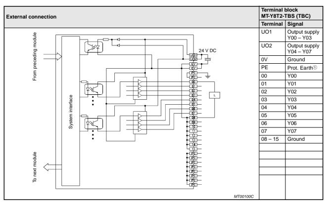
Tab. 10-18: External connection of the MT-Y8T2 module
