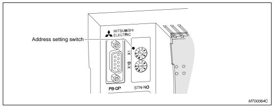
Fig. 6-1: Address setting switch
