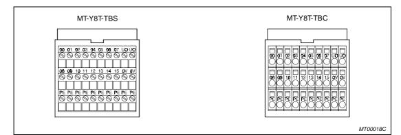
Fig. 4-14: Terminal blocks MT-Y8T-TBS and MT-Y8T-TBC
