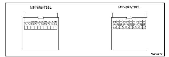
Fig. 4-23: Terminal blocks MT-Y8R5-TBS and MT-Y8R5-TBC
