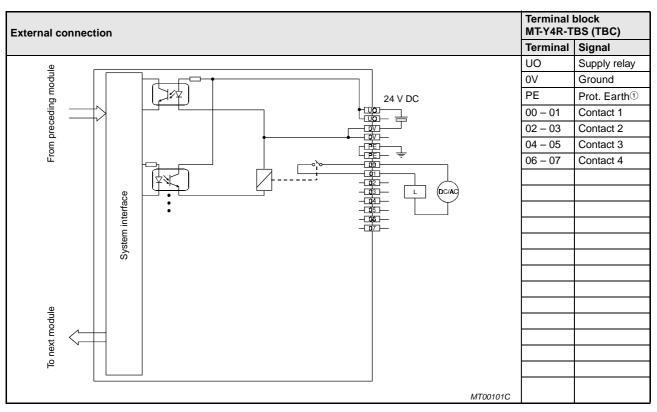
Tab. 10-20: External connection of the MT-Y4R module
