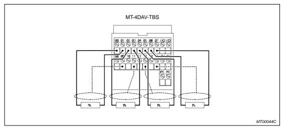
Fig. 4-46: Sample connection for voltage output
