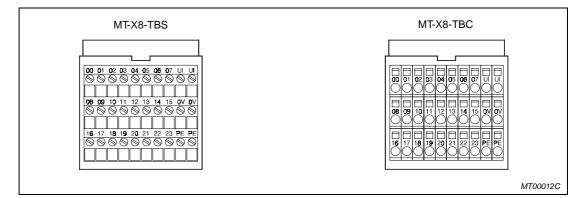
Fig. 4-8: Terminal blocks MT-X8-TBS and MT-X8-TBC
