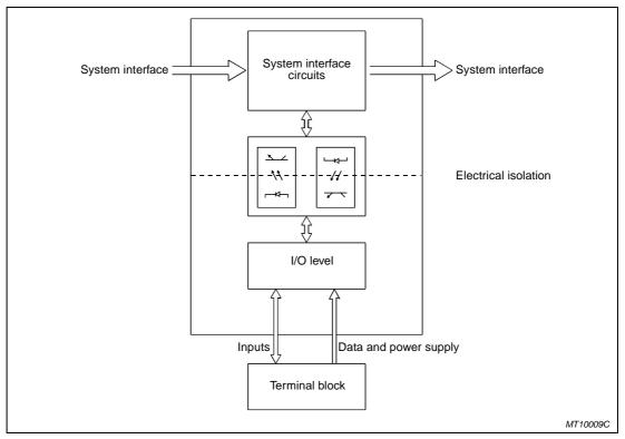
Fig. 4-3: Block diagram of the digital inputs of the MT-DP12E module
