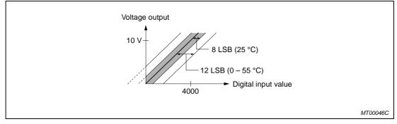
Fig. 4-48: Overall accuracy of the voltage output characteristics
