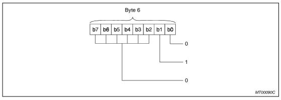
Fig. 9-9: Byte 6 of the diagnostics frame
