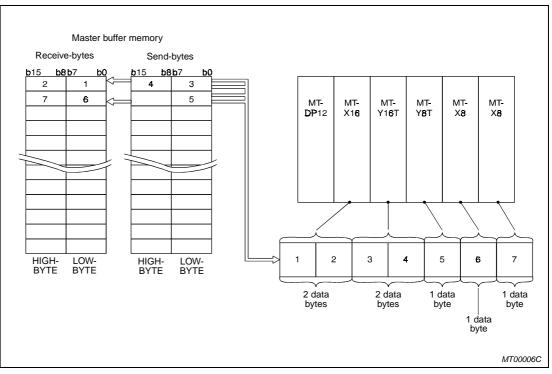
Fig. 3-7: Correct installation order
