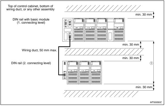
Fig. 5-3: Serial arrangement of the modules.
