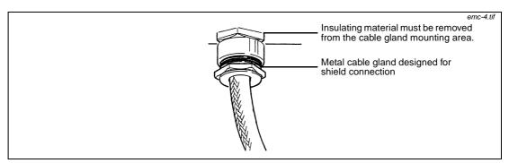
Abb. 5-12: Cable routing and shielding via metal cable gland
