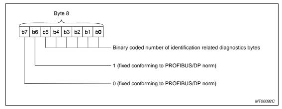
Fig. 9-11: Byte 8 of the diagnostics frame
