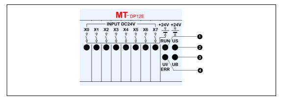
Fig. 9-3: Diagnostics indicators on the MT-DP12E module
