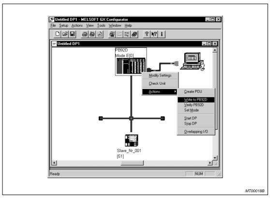
Fig. 7-18: Writing the parameterizing data
