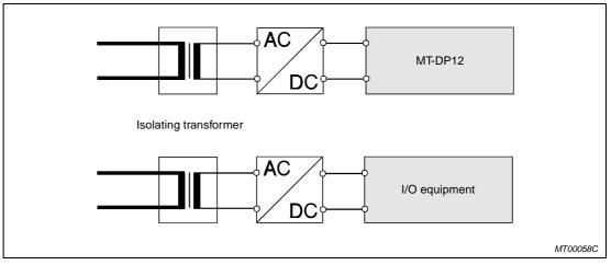
Fig. 5-15: Connection of an isolating transformer
