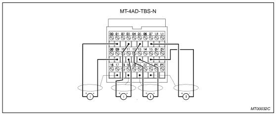
Fig. 4-34: Sample connection for current measurement
