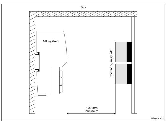
Fig. 5-5: Opposite arrangement of modules and equipment
