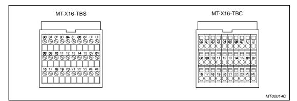
Fig. 4-10: Terminal blocks MT-X16-TBS and MT-X16-TBC
