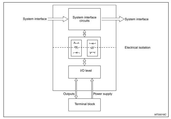
Fig. 4-12: Block diagram of the digital output modules
