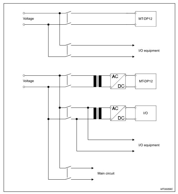
Fig. 5-16: Separation of the mains supply circuits
