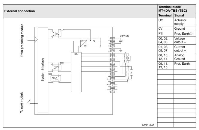
Tab. 10-30: External connection of the MT-4DA module
