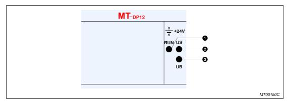
Fig. 9-2: Diagnostics indicators on the MT-DP12 module
