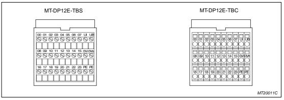
Fig. 4-5: Terminal blocks MT-DP12E-TBS and MT-DP12E-TBC
