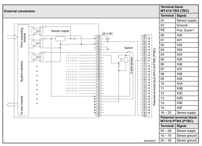
Tab. 10-12: External connection of the MT-X16 module
