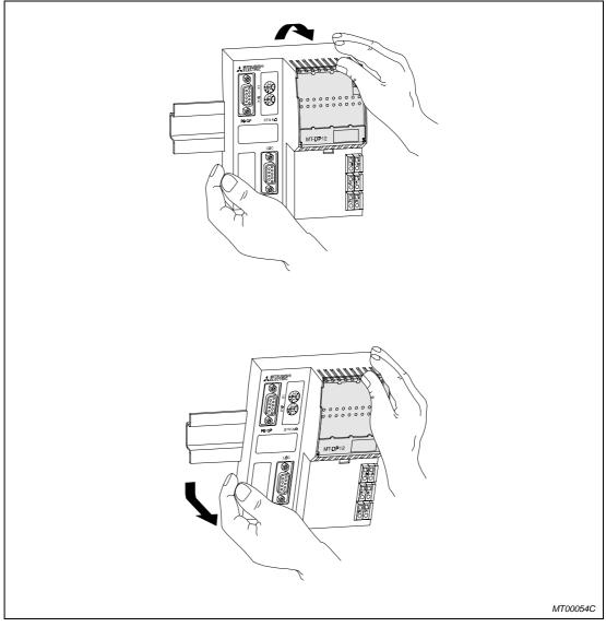
Fig. 5-7: Removal of a module
