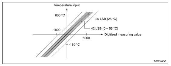
Fig. 4-42: Overall accuracy of the temperature input characteristics
