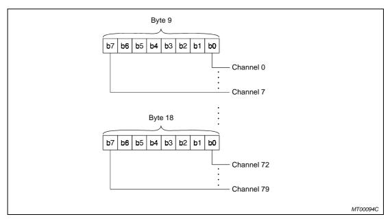
Fig. 9-12: 1st and 10th data byte of the identification related diagnostics
