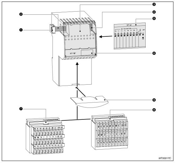
Fig. 4-13: Digital output module MT-Y8T
