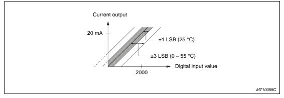
Fig. 4-56: Overall accuracy of the current output characteristics 0 – 20 mA
