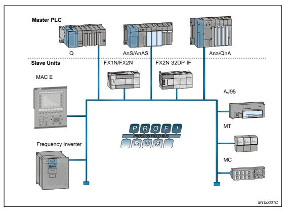
Fig. 3-1: System configuration PROFIBUS/DP
