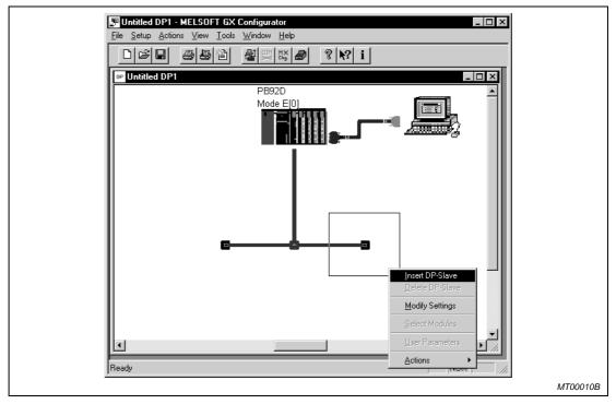
Fig. 6-9: Inserting the DP-slave
