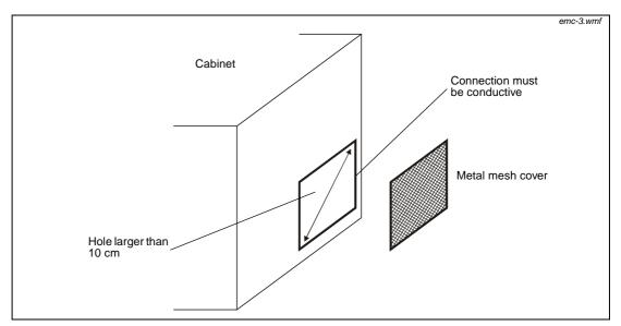
Abb. 5-11: Example for metal mesh cover
