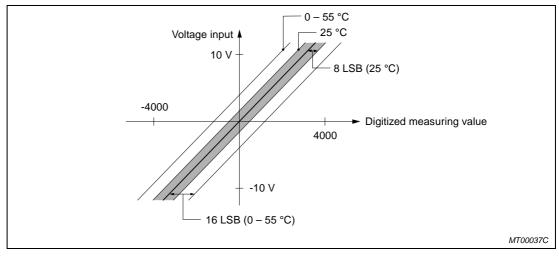
Fig. 4-39: Overall accuracy of the voltage input characteristics
