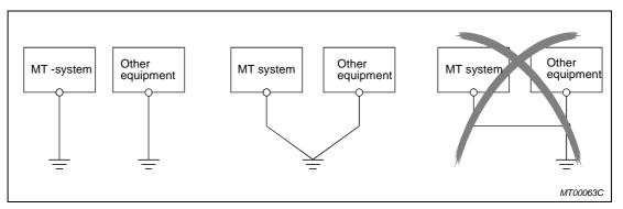
Fig. 5-18: Grounding connection
