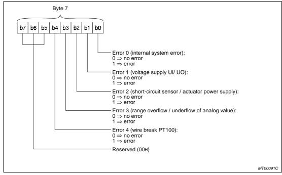
Figure 9-10 shows the assignment of bits to the according error codes:
