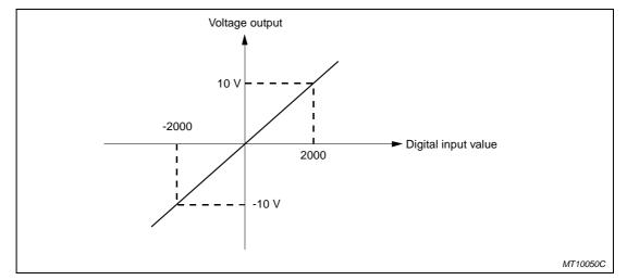
Fig. 4-52 shows the graph of the voltage output characteristics:
