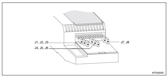
Fig. 4-30: Selection of measuring range via jumpers
