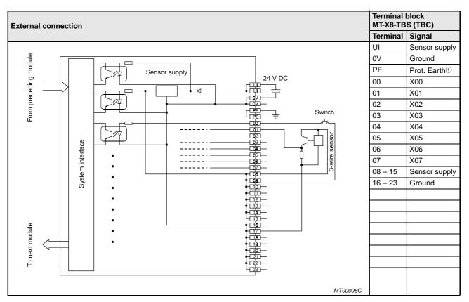
Tab. 10-10: External connection of the MT-X8 module
