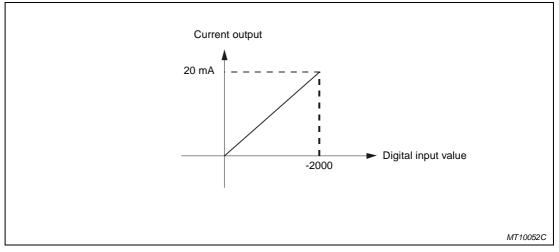
Fig. 4-54: Current output characteristics (0 – 20 mA)
