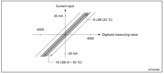
Fig. 4-40: Overall accuracy of the current input characteristics (±20 mA)
