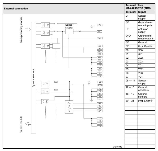
Tab. 10-24: External connection of the MT-X4Y4T module
