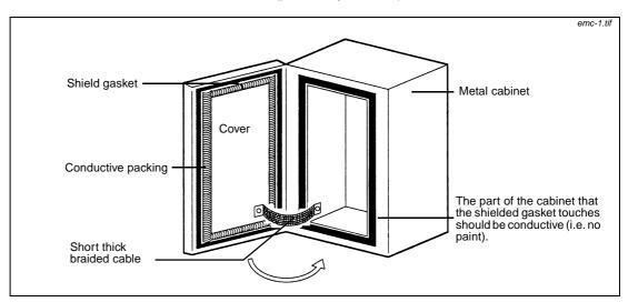
Abb. 5-10: Recommended design of a cabinet
