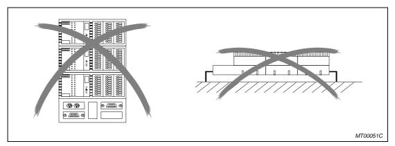
Fig. 5-4: Vertical and horizontal mounting not allowed
